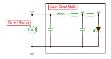
Consider the fact that a high speed current source results in a fast transient of the current to the load. Now if the load involves some inductivity in series, then the voltage drop across the inductive element will be given by
