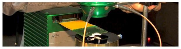
In this case, a 4cm broad strip line of 1.6mm thickness (standard circuit board) with 10cm length introduces an inductivity of 4.3nH which is approximately the value used in the example calculation on page 1 of this note.
