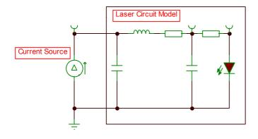
A SPICE<sup>3</sup> analysis of this circuit using an ideal current source generating an ideal step transient output results in the following current response through the light emitting semiconductor element.
