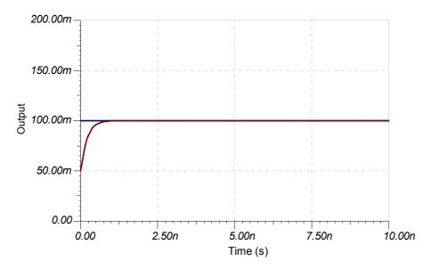
The analysis shows a fast, clean rise to the steady state with no overshoot. The transient response is found to be essentially due to the shunt capacitances – as to be expected from an ideal current source.
