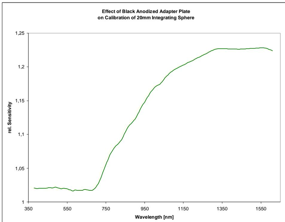
Artifex Engineering has addressed this issue by designing fibre port adapters which reflect so little light back into the integrating sphere that the miscalibration is less than 1% when the adapter plate is mounted. This is depicted in the following graph. Note the scale change when comparing the two graphs.
