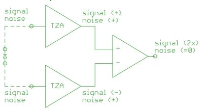
With the single ended input stage, any common mode noise introduced at the distal end of the cable is amplified by the input stage. The differential amplifier on the other hand amplifies only the signals which are generated by the source – in this case a photodiode. Common mode noise introduced at the photodiode, for example pickup from a motor or a transformer near the source, is subsequently eliminated in the differential stage following the transimpedance inputs.
