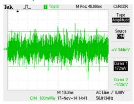
If the full speed of the amplifier is not required, a further noise reduction can be obtained by selecting a reduced bandwidth. This feature is available in the software of the TZA500. The following screen shots show signals from the same setup but with the bandwidth reduced to 100Hz.
