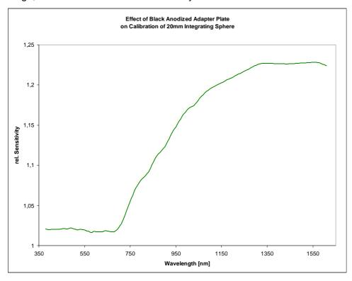
Artifex Engineering has addressed this issue by designing fibre port adapters which reflect so little light back into the integrating sphere that the miscalibration is less than 1% when the adapter plate is mounted. This is depicted in the following graph. Note the scale change when comparing the two graphs.
